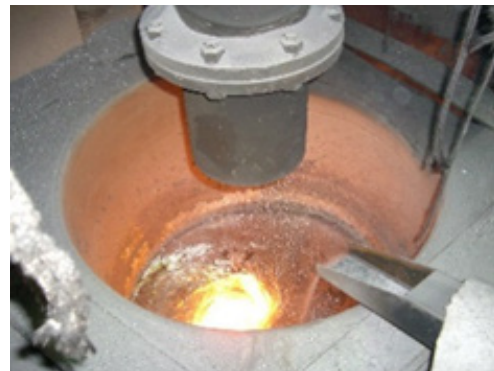
After: Pyrotek's LOTUSS system continuously melts scrap
